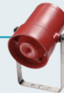
Alarm device DB3 Volume at 24 V and 1 m: 101... 115 dB Ex classification: II 2 G Ex d IIC T5 (-20 °C ≤ Ta ≤ 55 °C) Protection category: IP66/67 Order no.: BPZ:5757970001
